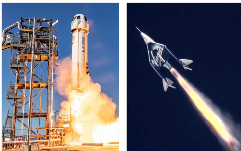
Figure 1 Suborbital spacecraft. Blue Origin's 'New Shepard' (left) uses a reusable rocket to launch a crew capsule that lands via parachute (photo credit: Blue Origin). Virgin Galactic's 'SpaceShipTwo' spaceplane (right) is launched from a carrier aircraft and lands as a glider (photo credit: Virgin Galactic).
